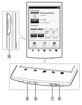
6 Charge/Busy indicator 7 ⊕ (Power) button 8 ⊈ Micro USB connector 9 RESET button 10 microSD card slot
