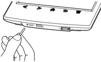
Press the RESET button with a small pin or clip. The screen will freeze; the Reader will not restart automatically.
